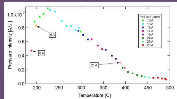
Graph showing the inverse temperature vs permeation rate of the data taken when the nichrome wire heater was cooled down from 500°C
