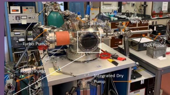
Two chambers separated by a holding pipe with a 1cm diameter palladium foil sealed in between two mini-conflats. Chambers pumped down to 10<sup>-8</sup> torr
